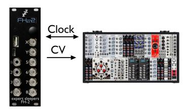
The FH-2 can operate as the clocking centre of your modular, also generating (syncable) LFOs, with no USB connection.
