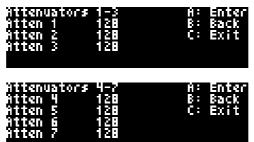
Each of the seven CV inputs has an attenuator control, which can be used to lower the range of strong input CVs to one more appropriate to the controlled parameter.
