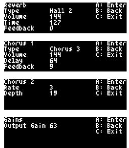
All modes offer two global audio effects, Reverb and Chorus, though both can in fact offer a wider range of effects than the name suggests. The synthesizer voices have independent effects sends to these two effects processes, and indeed the drum parts have per-drum settings for reverb and chorus depth.
