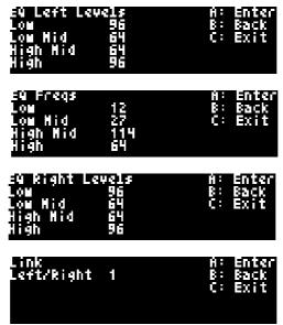
All modes offer global EQ settings. The left and right audio channels have independent EQ cut/boost controls, which can be linked (which they are by default).
