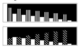
Pressing 'D' again changes to an editing mode where you are editing the even and odd harmonics in groups. Again, turning 'A' adjusts the current (group) level or slope. Turning 'B' chooses between the fundamental, the even harmonics, the odd harmonics, the even slope, and the odd slope.
