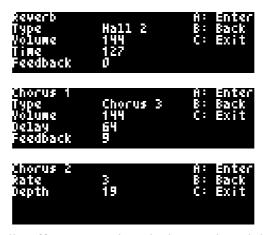
All modes offer two global audio effects, Reverb and Chorus, though both can in fact offer a wider range of effects than the name suggests. The synthesizer voices have independent effects sends to these two effects processes, and indeed the drum parts have per-drum settings for reverb and chorus depth.
