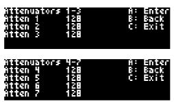
Each of the seven CV inputs has an attenuator control, which can be used to lower the range of strong input CVs to one more appropriate to the controlled parameter.
