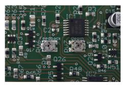
"RV6", marked "Feedback", scales the depth of the feedback control. It is factory-trimmed so that the feedback control turned fully clockwise doesn't quite send the module into self-oscillation.
