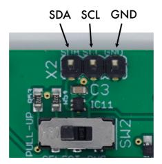
Make or remove I2C connections with the power off.
