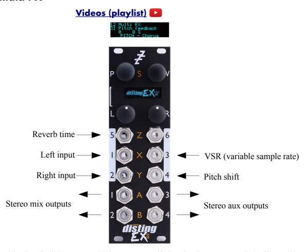
This algorithm is a flexible stereo multi-fx processor, offering simultaneous EQ, pitch effects, delay and reverb<sup>40</sup>. It also supports a "variable sample rate" feature, allowing you to change (under CV control if desired) the DSP's internal sample rate, which has a number of creative applications.
