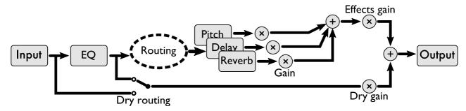
The routing between effects sections is quite flexible, allowing them to be chained in different orders, or to work in parallel.
