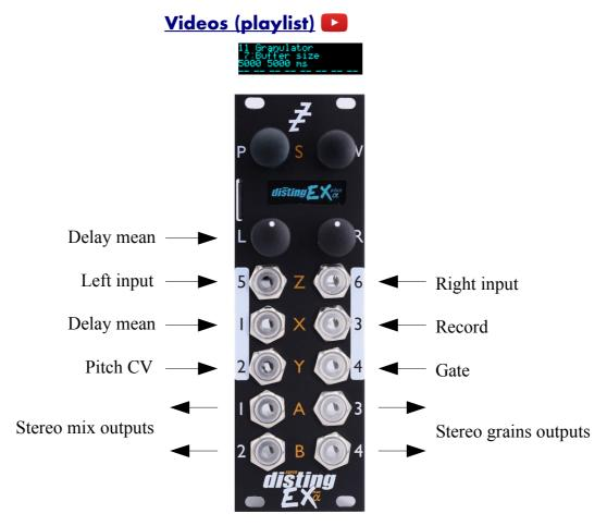
This algorithm implements a granular synthesis<sup>39</sup> engine, taking as its source material either live audio input or audio loaded from the SD card.
