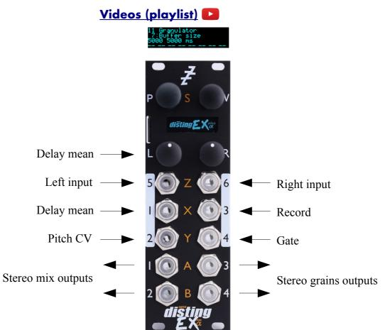
This algorithm implements a granular synthesis<sup>43</sup> engine, taking as its source material either live audio input or audio loaded from the SD card.
