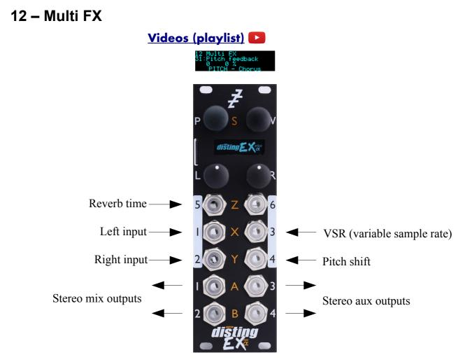
This algorithm is a flexible stereo multi-fx processor, offering simultaneous EQ, pitch effects, delay and reverb<sup>44</sup>. It also supports a "variable sample rate" feature, allowing you to change (under CV control if desired) the DSP's internal sample rate, which has a number of creative applications.
