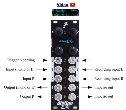
This algorithm is performs real-time <u>convolution</u><sup>49</sup> of the input signal and another signal (often called an 'impulse response') which can be loaded from the MicroSD card or recorded live into the module's memory.
