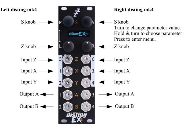
We do not propose to reproduce the entire disting mk4 <u>user manual</u><sup>8</sup> here, which is itself a 118 page document. Instead, below is a list of ways in which the disting EX in dual mode differs from a disting mk4.
