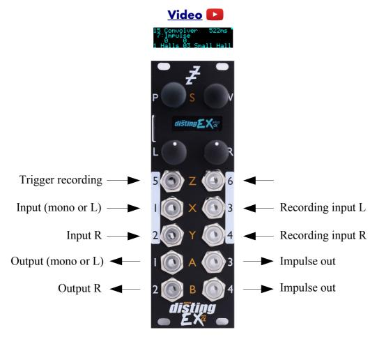
This algorithm performs real-time <u>convolution</u><sup>49</sup> of the input signal and another signal (often called an 'impulse response') which can be loaded from the MicroSD card or recorded live into the module's memory.
