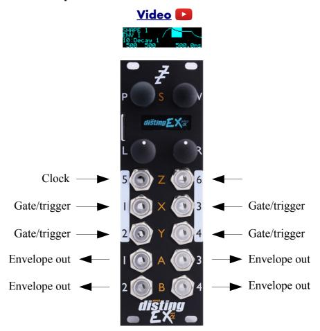
This algorithm is a quad complex (DAHDSR) envelope generator, with optional VCA functionality. Various trigger modes include gated, triggered (one-shot) and looping.
