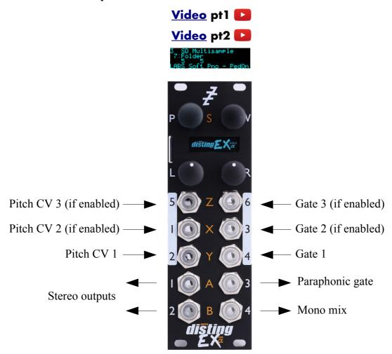
The SD Multisample algorithm is an 8 voice polyphonic sample playback instrument, playing WAV files from the MicroSD card. It can have up to 3 input CV/gate pairs, or can be played via MIDI. It supports both velocity switches and round robins per sample.
