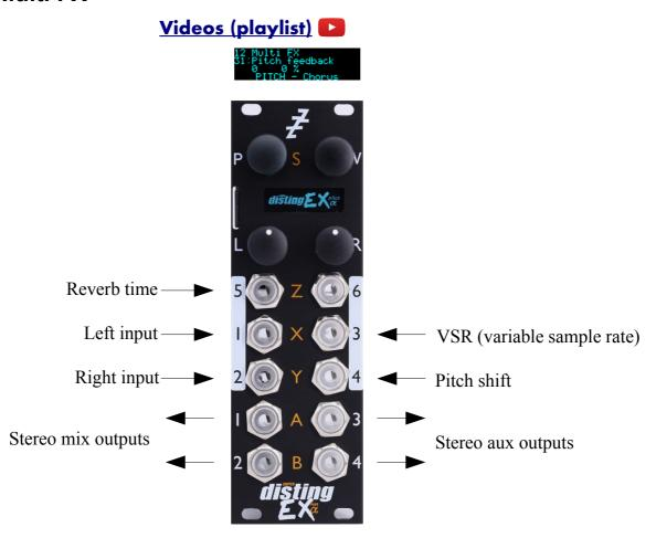
This algorithm is a flexible stereo multi-fx processor, offering simultaneous EQ, pitch effects, delay and reverb<sup>44</sup>. It also supports a "variable sample rate" feature, allowing you to change (under CV control if desired) the DSP's internal sample rate, which has a number of creative applications.
