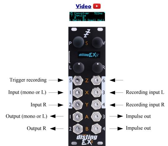
This algorithm performs real-time <u>convolution</u><sup>49</sup> of the input signal and another signal (often called an 'impulse response') which can be loaded from the MicroSD card or recorded live into the module's memory.
