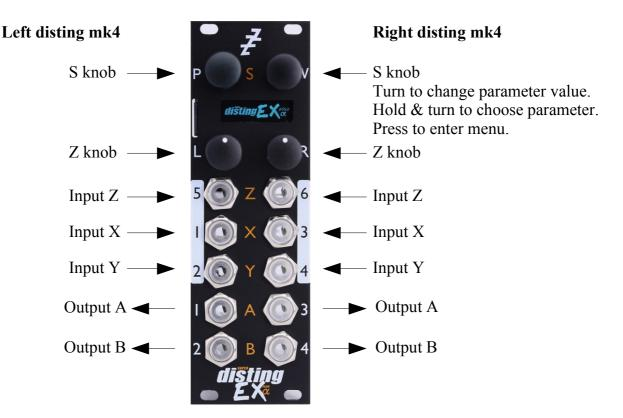
We do not propose to reproduce the entire disting mk4 <u>user manual</u><sup>8</sup> here, which is itself a 123 page document. Instead, below is a list of ways in which the disting EX in dual mode differs from a disting mk4.
