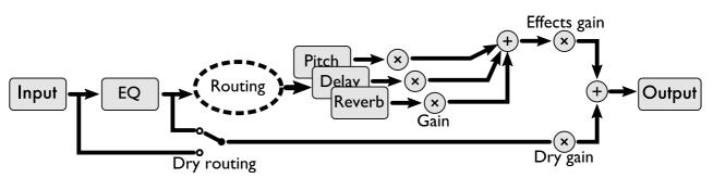
The routing between effects sections is quite flexible, allowing them to be chained in different orders, or to work in parallel.
