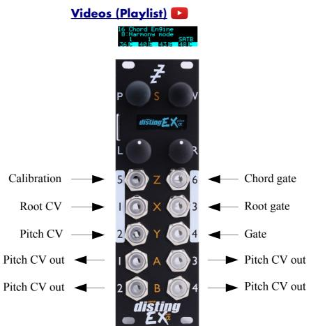
This algorithm generates chords of pitch CVs from an input pitch CV, with a number of options for how the harmony CVs are worked out.
