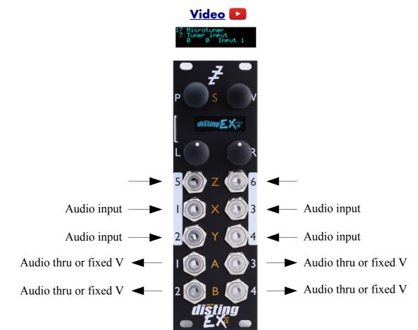
This algorithm is a tuner, displaying the pitch of up to four input signals at once.
