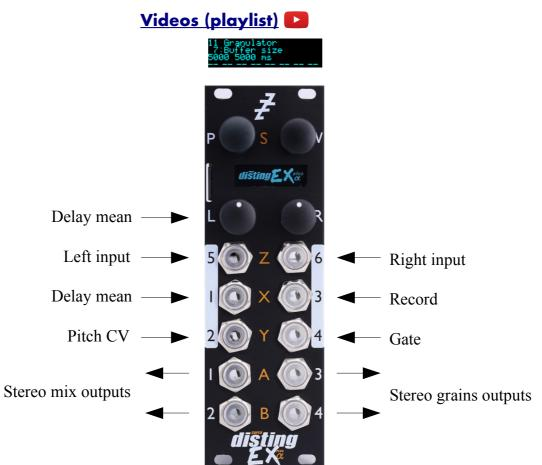
This algorithm implements a granular synthesis<sup>44</sup> engine, taking as its source material either live audio input or audio loaded from the SD card.
