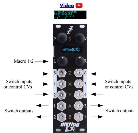
This algorithm offers six highly configurable sequential or voltage controlled switches. Being DC-coupled, it can switch audio or CVs.
