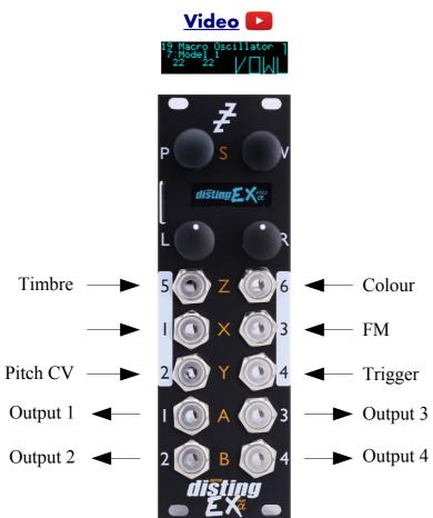
This algorithm is an implementation of the open source <u>Braids</u><sup>60</sup> module by Émilie Gillet. It provides four independent instances of the module, each with its own output. The disting EX's inputs can be freely assigned to any or all of the instances. Control via MIDI is also possible, making this an excellent application for the <u>CVM-8</u><sup>61</sup> module to provide, say, separate trigger inputs for all four instances.
