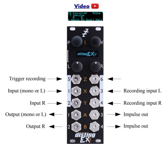
This algorithm performs real-time <u>convolution</u><sup>50</sup> of the input signal and another signal (often called an 'impulse response') which can be loaded from the MicroSD card or recorded live into the module's memory.
