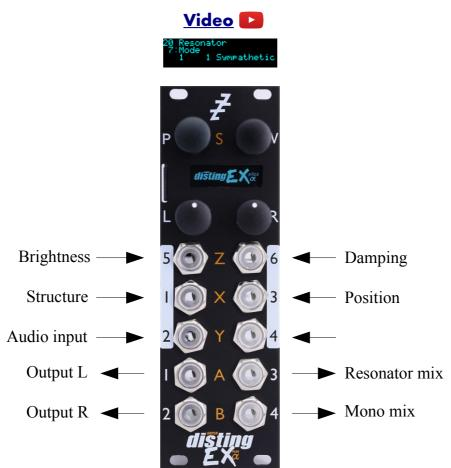
This algorithm is an implementation of the open source <u>Rings</u><sup>64</sup> module by Émilie Gillet.
