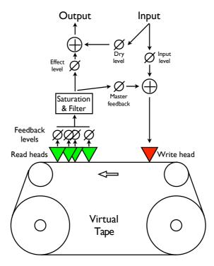
There are four 'tape read heads' with independent delay times and stereo positions, allowing for straight stereo delays, ping pong delays, or hybrid multi-tap style effects.
