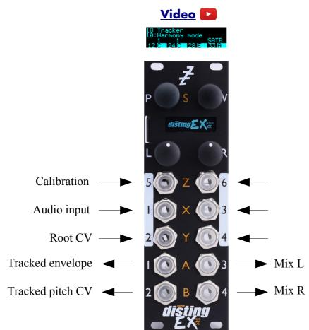
This algorithm tracks the pitch and envelope of an audio signal, and uses it to generate either CVs (of the tracked pitch and a chord related to it) or pitch-shifted versions of the input audio to form a chord.
