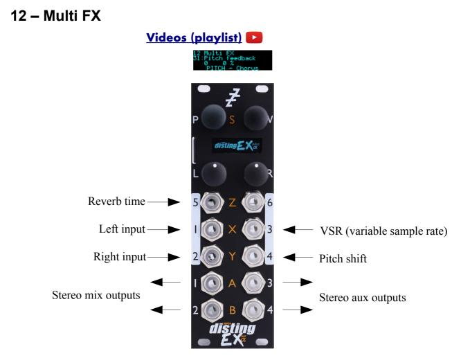
This algorithm is a flexible stereo multi-fx processor, offering simultaneous EQ, pitch effects, delay and reverb<sup>45</sup>. It also supports a "variable sample rate" feature, allowing you to change (under CV control if desired) the DSP's internal sample rate, which has a number of creative applications.
