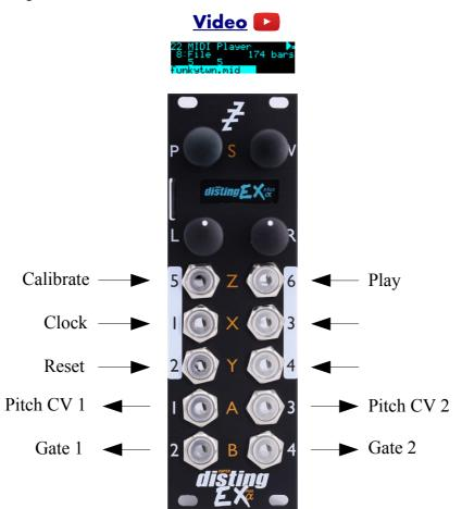
This algorithm plays standard MIDI files, outputting the MIDI via the breakout, and converting the MIDI to CVs and gates. It will use an internal clock (using the file's tempo, if specified), or sync to analogue clocks or incoming MIDI clock.
