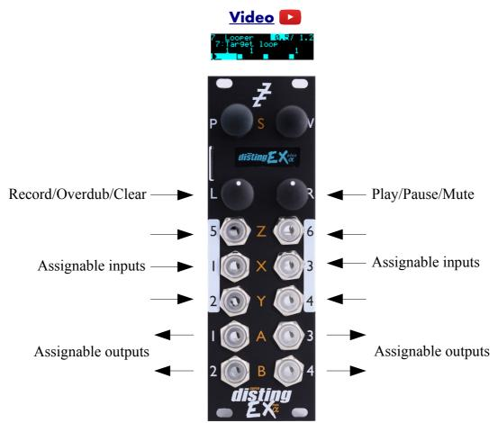
This algorithm provides four simultaneous loopers, with two button record/play/overdub control in the manner of many stomp-box loopers.
