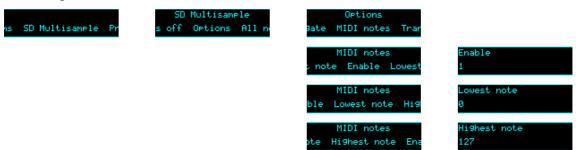
The 'Delay time' parameter can optionally follow MIDI clock. This is also enabled via the menu:
