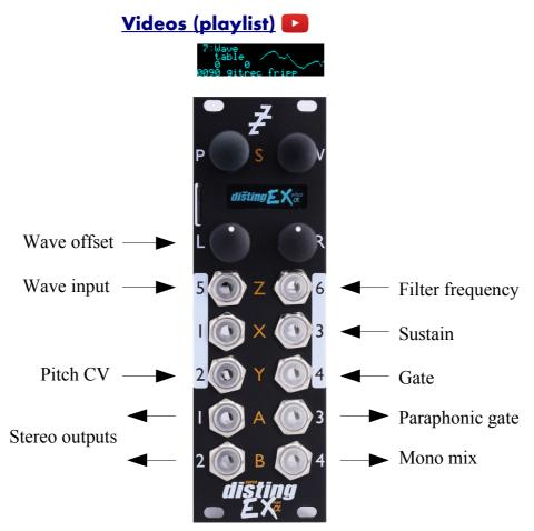
This algorithm is a complete 8 voice polyphonic synthesizer, using wavetable oscillators. Each voice has two envelopes, a filter and an LFO. Delay and chorus effects are also provided.
