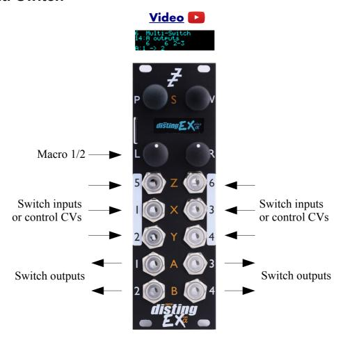
This algorithm offers six highly configurable sequential or voltage controlled switches. Being DC-coupled, it can switch audio or CVs.
