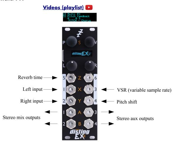
This algorithm is a flexible stereo multi-fx processor, offering simultaneous EQ, pitch effects, delay and reverb<sup>45</sup>. It also supports a "variable sample rate" feature, allowing you to change (under CV control if desired) the DSP's internal sample rate, which has a number of creative applications.
