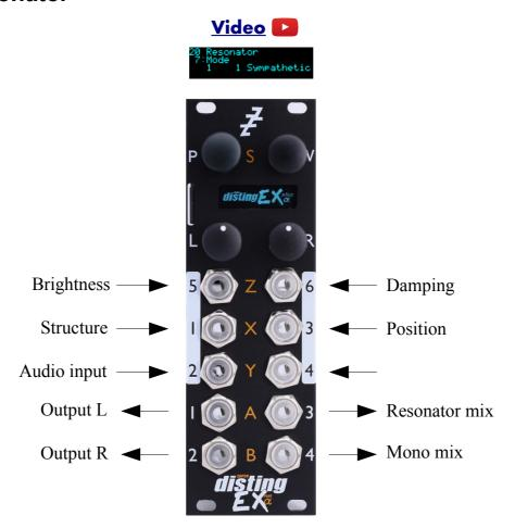
This algorithm is an implementation of the open source Rings<sup>64</sup> module by Émilie Gillet.
