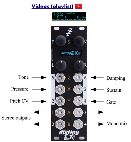
This algorithm is an 8 voice polyphonic synthesizer, based on the method of exciting a resonant structure with a burst of audio. It produces results than can sound like a stringed instrument being plucked/struck.
