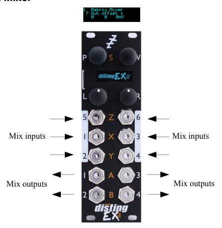
The Matrix Mixer is a flexible 6 into 4 mixer, mainly designed for CV processing, though it will happily handle audio as well. As well as a static mix, the algorithm is capable of complex dynamic mixes when CV mapping is used, and also of CV generation – for example, by automating the input and output offsets to generate four CVs which might control the rest of your patch in a 'macro' fashion.
