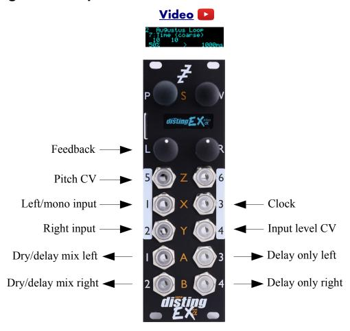
Augustus Loop is a disting EX implementation of one of Expert Sleepers' oldest products, the VST plug-in of the same name (<u>here</u><sup>18</sup>). Essentially, it's a tape-inspired stereo delay.
