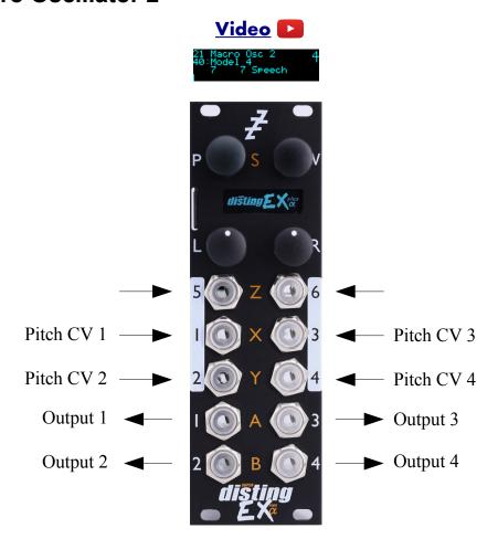
This algorithm is an implementation of the open source <u>Plaits</u><sup>66</sup> module by Émilie Gillet. It provides four independent instances of the module. The disting EX's inputs can be freely assigned to any or all of the instances. Control via MIDI is also possible, making this an excellent application for the <u>CVM-8</u><sup>67</sup> module to provide, say, separate trigger inputs for all four instances.
