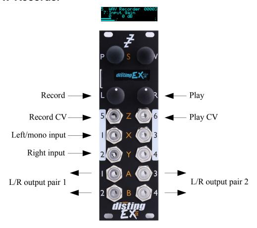
This algorithm records audio (or CV) to the MicroSD card as a WAV file. It can record up to six channels of audio at 48 or 96kHz, 16 or 24 bit. It can also play previous recordings, though the various WAV playing algorithms offer many more possibilities.
