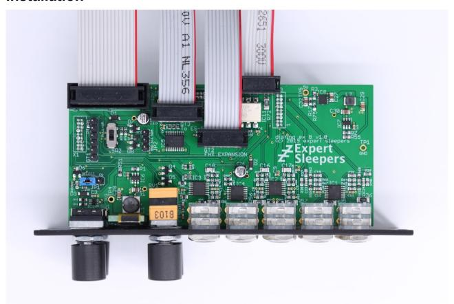
House the module in a Eurorack case of your choosing. The power connector is 16-pin <u>Doepfer standard</u><sup>2</sup>. If using the power cable supplied with the module, the red edge of the cable is furthest from the top edge of the PCB, and carries -12V. ("-12V" is marked on the PCB itself next to this end of the connector.) Be sure to connect the other end of the power cable correctly, again so -12V corresponds to the red stripe on the cable.
