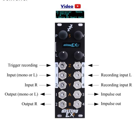
This algorithm performs real-time <u>convolution</u><sup>50</sup> of the input signal and another signal (often called an 'impulse response') which can be loaded from the MicroSD card or recorded live into the module's memory.
