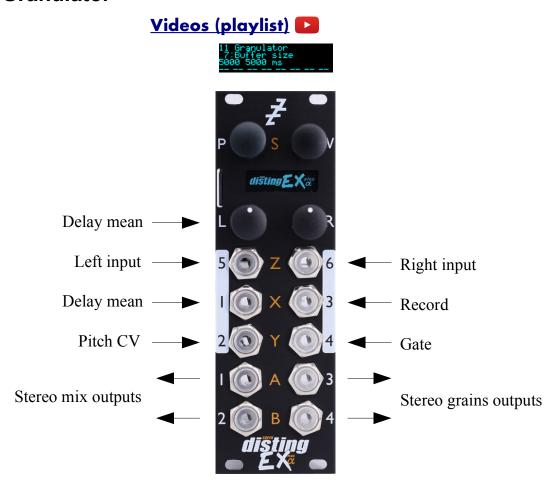
This algorithm implements a granular synthesis<sup>44</sup> engine, taking as its source material either live audio input or audio loaded from the SD card. Live audio can be recorded into a buffer (maximum size about 31 seconds) or streamed continuously.
