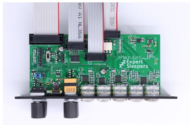
House the module in a Eurorack case of your choosing. The power connector is 16-pin <u>Doepfer</u> <u>standard</u><sup>2</sup>. If using the power cable supplied with the module, the red edge of the cable is furthest from the top edge of the PCB, and carries -12V. ("-12V" is marked on the PCB itself next to this end of the connector.) Be sure to connect the other end of the power cable correctly, again so -12V corresponds to the red stripe on the cable.
