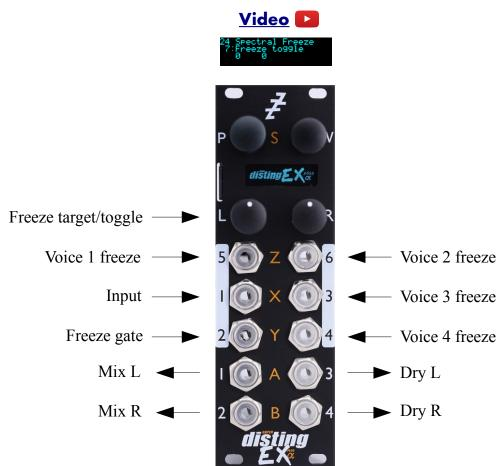
This algorithm is an audio 'freeze' effect – it captures sound at a moment in time and sustains it indefinitely. The 'spectral' part of the name indicates that it works in the frequency domain – unlike simple loopers or granular effects, which work in the time domain, this algorithm captures the spectrum of a sound (using an FFT) and uses that to resynthesize audio<sup>77</sup>.
