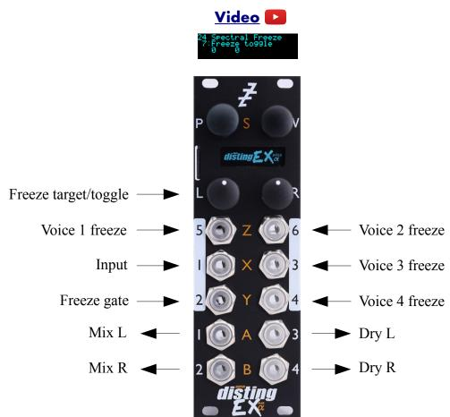
This algorithm is an audio 'freeze' effect – it captures sound at a moment in time and sustains it indefinitely. The 'spectral' part of the name indicates that it works in the frequency domain – unlike simple loopers or granular effects, which work in the time domain, this algorithm captures the spectrum of a sound (using an FFT) and uses that to resynthesize audio<sup>78</sup>.
