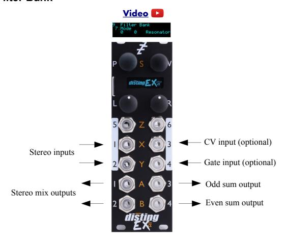
This algorithm provides a bank of eight parallel stereo bandpass filters or resonators. The filters' levels can be controlled manually, via CV, or with envelopes driven from gates, and their pitch can also be set manually or via CV or MIDI. An internal octature LFO is also provided for the levels.
