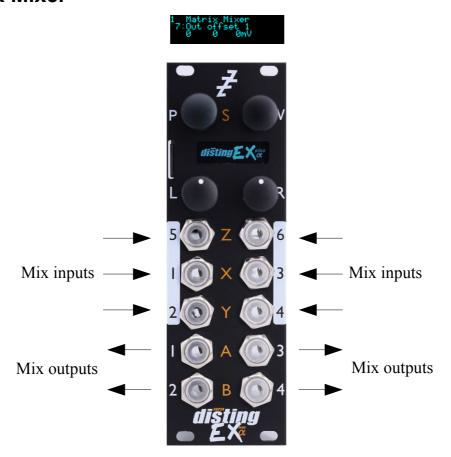
The Matrix Mixer is a flexible 6 into 4 mixer, mainly designed for CV processing, though it will happily handle audio as well. As well as a static mix, the algorithm is capable of complex dynamic mixes when CV mapping is used, and also of CV generation – for example, by automating the input and output offsets to generate four CVs which might control the rest of your patch in a 'macro' fashion.
