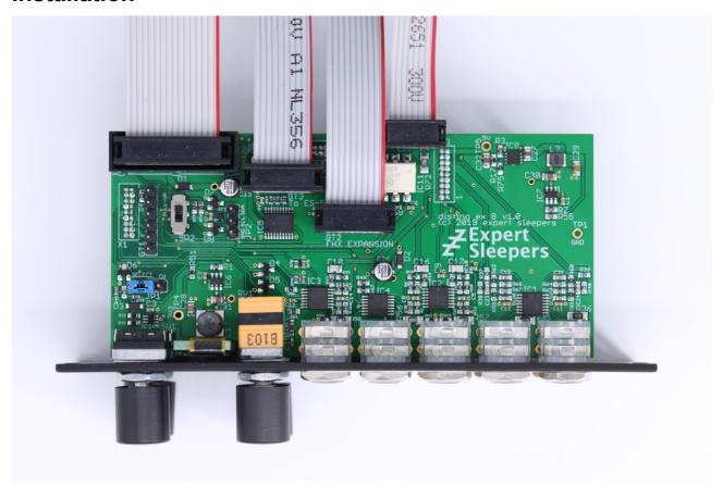
House the module in a Eurorack case of your choosing. The power connector is 16-pin <u>Doepfer standard</u><sup>1</sup>. If using the power cable supplied with the module, the red edge of the cable is furthest from the top edge of the PCB, and carries -12V. ("-12V" is marked on the PCB itself next to this end of the connector.) Be sure to connect the other end of the power cable correctly, again so -12V corresponds to the red stripe on the cable.
