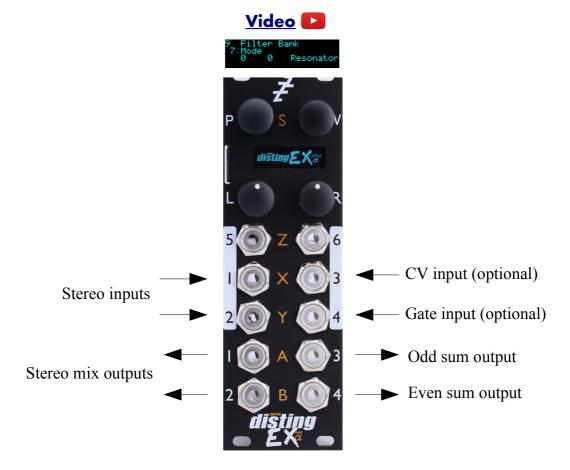
This algorithm provides a bank of eight parallel stereo bandpass filters or resonators. The filters' levels can be controlled manually, via CV, or with envelopes driven from gates, and their pitch can also be set manually or via CV or MIDI. An internal octature LFO is also provided for the levels.
