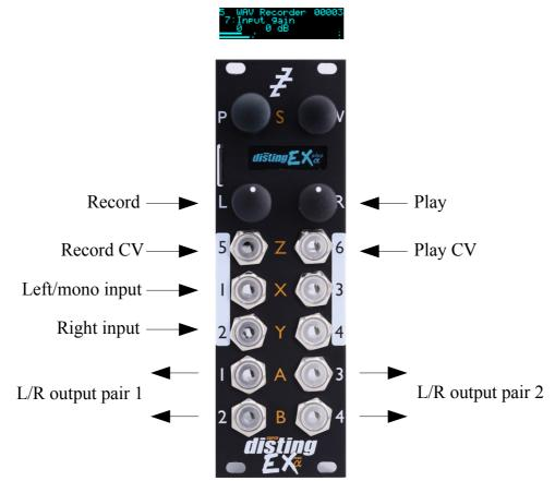
This algorithm records audio (or CV) to the MicroSD card as a WAV file. It can record up to six channels of audio at 48 or 96kHz, 16 or 24 bit. It can also play previous recordings, though the various WAV playing algorithms offer many more possibilities.
