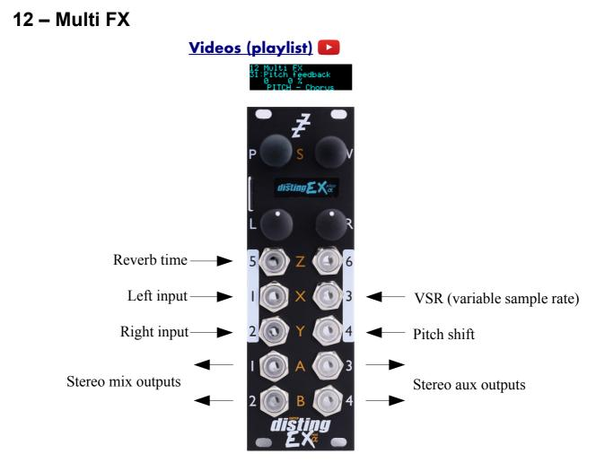
This algorithm is a flexible stereo multi-fx processor, offering simultaneous EQ, pitch effects, delay and reverb<sup>40</sup>. It also supports a "variable sample rate" feature, allowing you to change (under CV control if desired) the DSP's internal sample rate, which has a number of creative applications.
