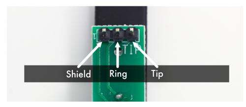
Use the jump cables to connect the relevant pins of the TRS sockets to the pins of the breakout headers on the disting NT that you would like to use.
