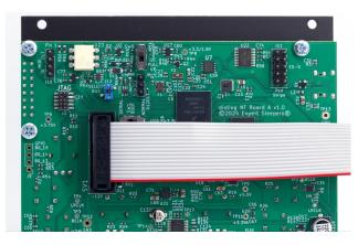
Please observe ESD (electro-static discharge) precautions when handling the module (and indeed, any module).
