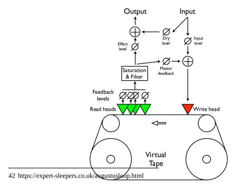
There are four 'tape read heads' with independent delay times and stereo positions, allowing for straight stereo delays, ping pong delays, or hybrid multi-tap style effects.
