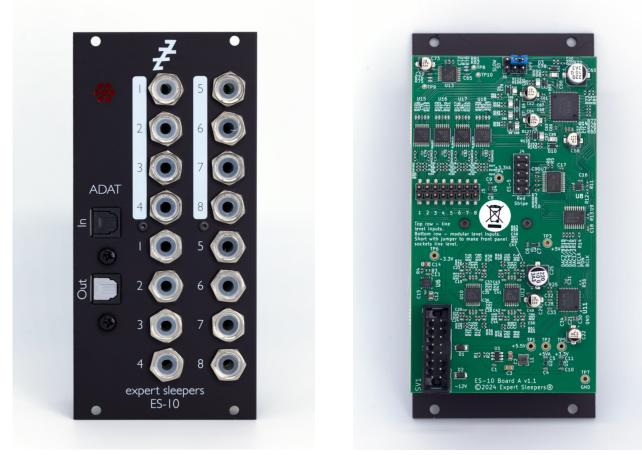
The ES-10 is a Eurorack 8-in/8-out ADAT interface, with DC-coupled inputs and outputs that can be used for both audio and CVs.
