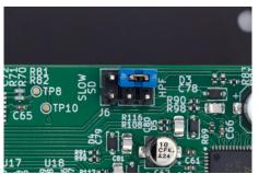
This actually equivalent to there being no jumper at all, since the top row of pins are simply ground.
