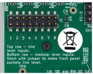
Instructions are printed on the PCB. Fitting a jumper across the pins for a particular input makes the front panel socket line level instead of modular level.
