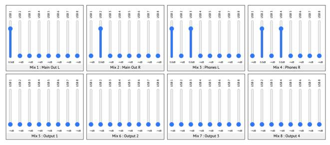
The eight 'Mix' boxes correspond to the eight outputs of the Mixer processing block above. Each mix, and each fader, is labelled with the input or output name as set in the routing controls.
