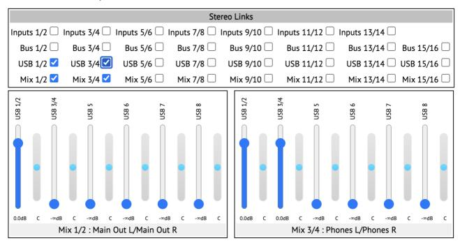
Note that we now have a single mixer shown for Mix 1/2, and a single mixer for Mix 3/4. Also, in the mixers, USB 1/2 and USB 3/4 each have a single fader controlling the two channels. Finally, since the mixers are now stereo, each channel has a pan control.
