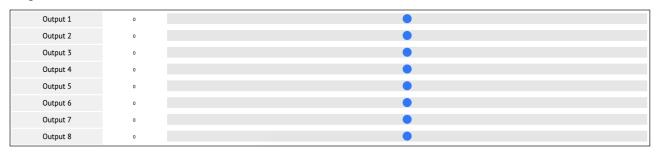
Internally this is implemented using the mixer hardware, so a mixer needs to be routed to any output to which you want to apply a DC offset.
