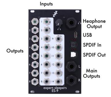
The ES-9 has fourteen analogue inputs on 3.5mm TS jack sockets. These are designed to cope with any Eurorack signal, and are DC coupled, so can be used for CVs as well as audio. An input voltage of approximately  $\pm 10$ V will give a 0 dBFS level in your DAW.
