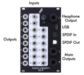
The ES-9 has fourteen analogue inputs on 3.5mm TS jack sockets. These are designed to cope with any Eurorack signal, and are DC coupled, so can be used for CVs as well as audio. An input voltage of approximately  $\pm 10$ V will give a 0 dBFS level in your DAW.
