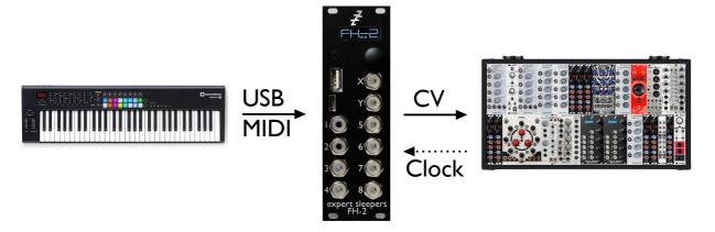
Up to 16 note polyphonic conversion, with optional pitch/gate/velocity etc. CVs per note. Also features arpeggiation, keyboard splits and more.
