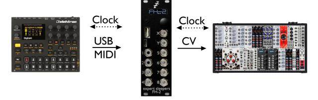
Multiple clock outs at different divisions, run/stop triggers etc. Groovebox, FH-2, or another module can be the clock master.
