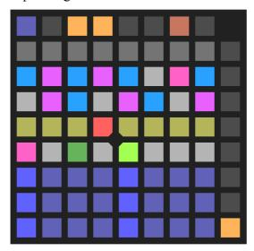
Rows 1-4 show all 32 steps of the lane. The current step is highlighted magenta. Steps within the start and end points are shown white (off) or green (on). As in the overview, pressing a button for a step toggles it on or off, and accents are set by holding button 7/9 and pressing the step button. Note that you can edit steps that are not within the start & end points (shown blue).
