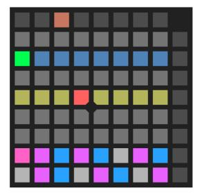
Row 7 controls the gate length, from short on the left to long on the right. Gate length is a percentage of the step time, except at value 0, where it becomes a fixed length trigger pulse.
