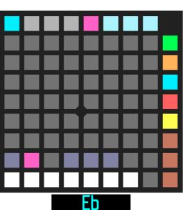
Holding button 9/3 (dark orange) activates 'nudge' mode, in which buttons 3/9 and 4/9 move the sequence one step to the left or right respectively.
