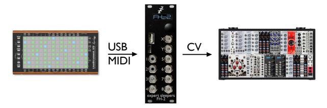
Up to 16 simultaneous touches converted with full position/pressure/glide etc. per touch.
