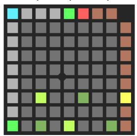
Steps proceed from left to right. As for the note sequencers, buttons 1/9 to 4/9 switch between pages of 8 steps. The current step, if it falls on the current page, is highlighted.
