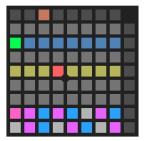
Row 7 controls the gate length, from short on the left to long on the right. Gate length is a percentage of the step time, except at value 0, where it becomes a fixed length trigger pulse.
