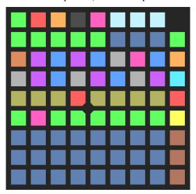
Row 8 controls the gate length, from short on the left to long on the right. As for the Euclidean patterns, gate length is a percentage of the step time, except at value 0, where it becomes a fixed length trigger pulse.
