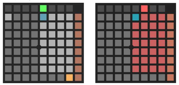
The 4x7 grid of white (load) or red (save) buttons represent the 28 sequence slots. The slot most recently accessed by the drum sequencer is indicated with a blue highlight. Pressing the button for a sequence slot loads or saves the drum sequencer's sequence from or to that slot.
