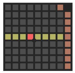
Currently the only global setting is a reset rate, analogous to that on each drum sequencer lane or note sequencer – it sets the number of quarter notes after which all eight drum lanes will reset to their first step. This is selected using 1/5 to 8/5 (yellow). The chosen value is shown in red; press the same button again to turn the reset feature off.
