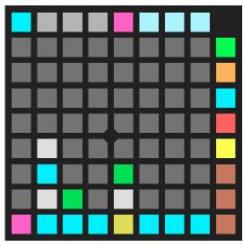
White indicates a step which is 'off'; blue indicates a standard step which is 'on'; yellow indicates a 'ratchet' step which is 'on'. Green indicates a tie. The current step is highlighted magenta.
