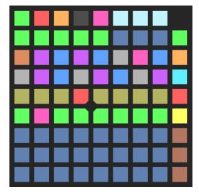
Row 8 controls the gate length, from short on the left to long on the right. As for the Euclidean patterns, gate length is a percentage of the step time, except at value 0, where it becomes a fixed length trigger pulse.
