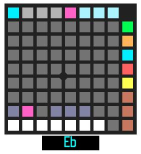
Holding button 9/3 (dark orange) activates 'nudge' mode, in which buttons 3/9 and 4/9 move the sequence one step to the left or right respectively.
