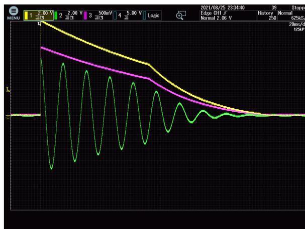
The yellow trace is the CV input; the magenta is the CV output. The green trace shows the module's audio output. In this image, the zero-cross feature is not enabled. Notice how the audio waveform rises extremely abruptly as the envelope opens. This would be audible as a nasty click. Worse, as the relative timings of the envelope and the sine wave change from note to note, the click will come and go randomly.
