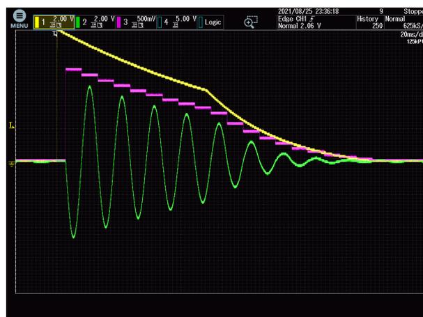
Notice how the output CV (magenta) is now stepped, and only changes when the audio passes through zero. Also, the output waveform no longer has the click at the start, since it remains at zero until the first zero-crossing.
