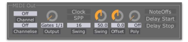
This section allows a Gate Expander output to be used as a MIDI output. Because the ES-4's outputs are derived from an audio signal, the MIDI messages sent from an ES-4 are free from the <u>timing problems</u> often associated with regular (e.g. USB) MIDI interfaces.
