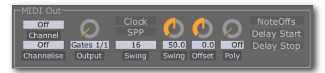
This section allows a Gate Expander output to be used as a MIDI output. Because the ES-5's outputs are derived from an audio signal, the MIDI messages sent from an ES-5 are free from the <u>timing problems</u> often associated with regular (e.g. USB) MIDI interfaces.
